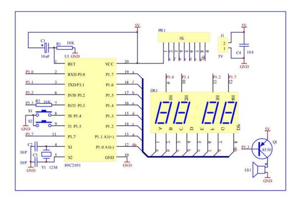
Note: there is direction for PR1 Resisters Packs , there is one side of the word in the direction of the MCU.Pay an attention!!!
